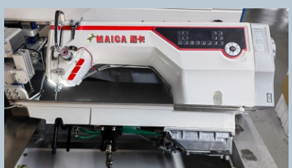
机头可翻倒 Sewing head to be turned over 方便维修和更换梭芯。 Easy for maintenance and changing bobbin.
