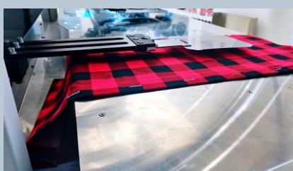
特制放料槽 Fabric notch area 针对长款口袋 Customized for large pocket
