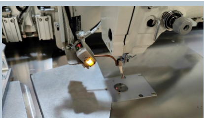
袋边精准识别:精准缝纫 Hemming edge sensing, accurate sewing
