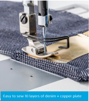
Easy to sew 10 layers of denim + copper plate
